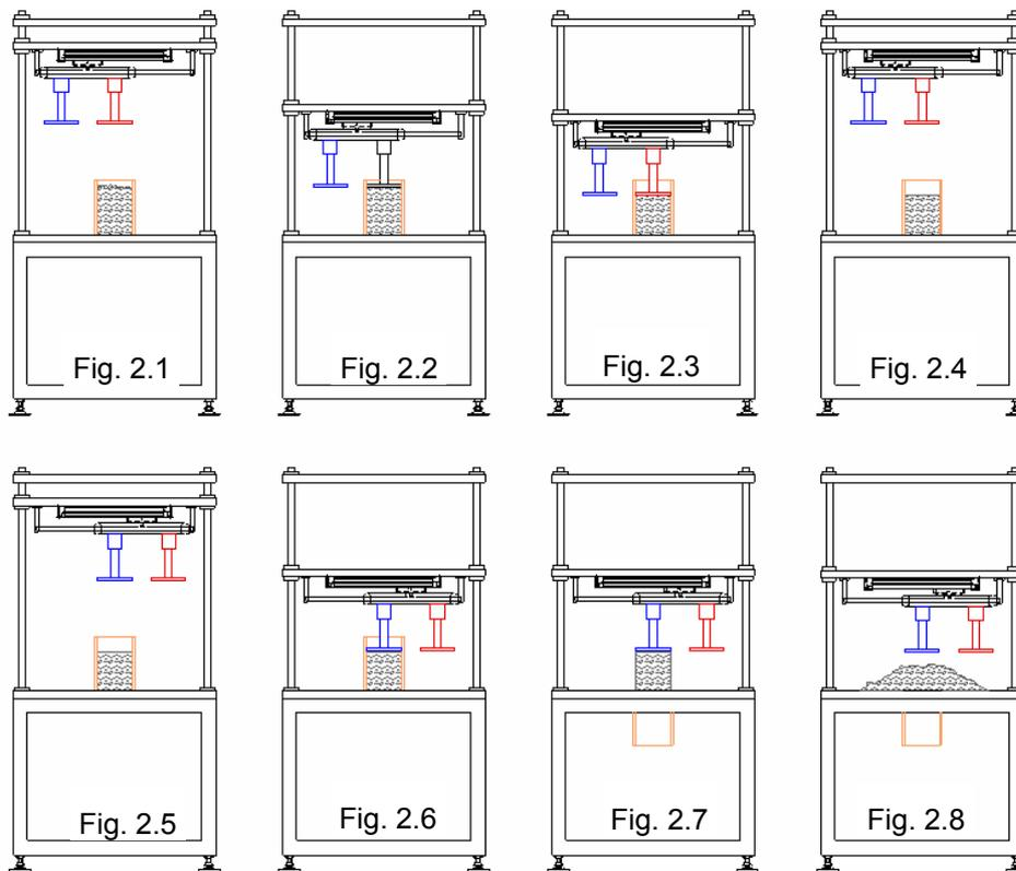
**Figures 2.1 to 2.8 Schematic of large coal tester**
