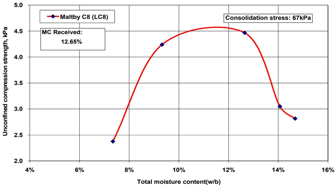
Figure 4.1 Stress-Moisture-Cohesion Function of Maltby C8
