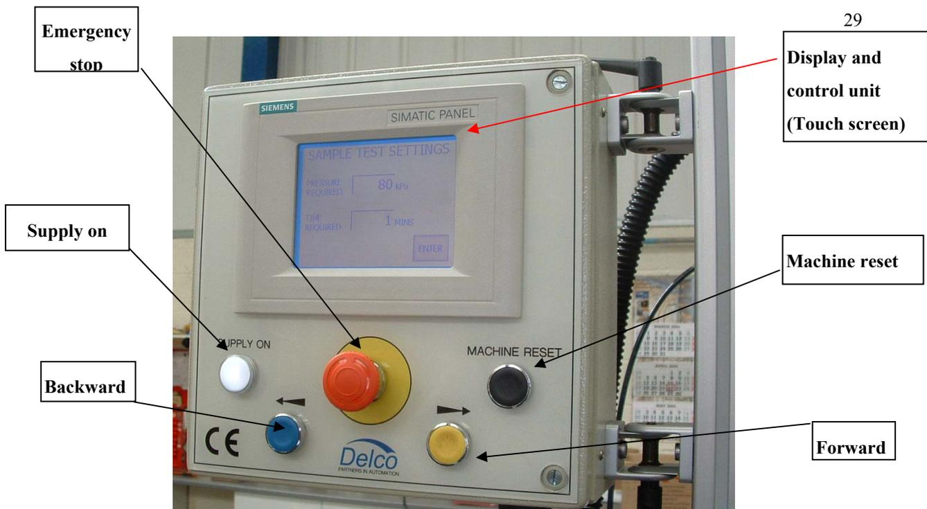
**Figure 5.3 Programmable control unit**
