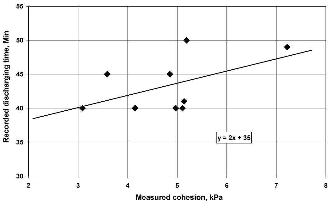
Figure 6.9 Discharging time vs mean cohesion of the consignment
