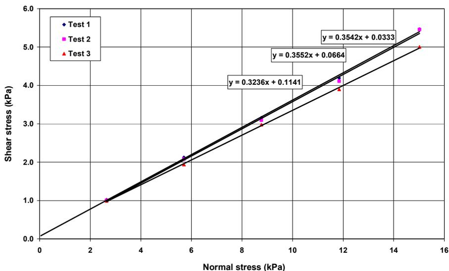
Figure 4.5 Shear stress vs. normal stress for dry coal on mild steel wall
