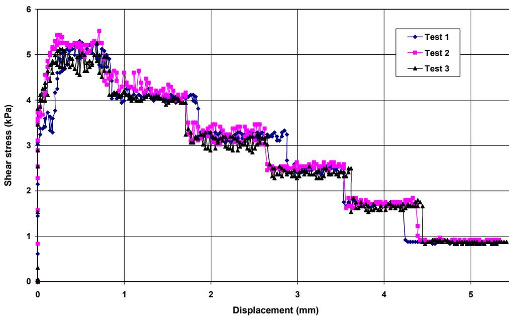
Figure 4.3 Shear stress vs. displacement for the dry coal on nedox treated wall
