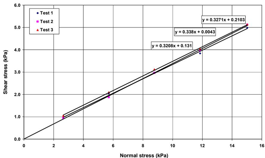
Figure 4.6 Shear stress vs. normal stress for dry coal on Mylar wall
