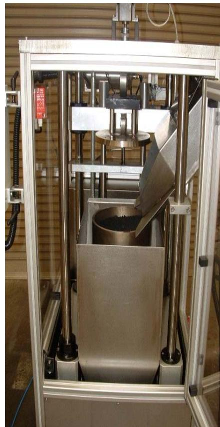
**Figure 5.2 Filling chute attached to the side of machine**
