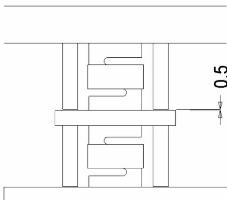
**Figure 2.10 Arrangement for loadcells**
