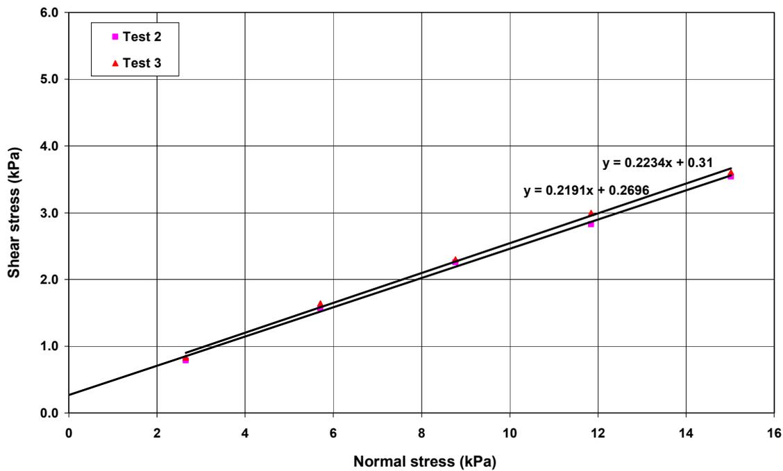
Figure 4.8 Shear stress vs. normal stress for wet coal on nedox treated wall
