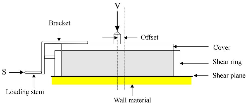
Figure 4.2 Jenike shear cell for wall friction test
