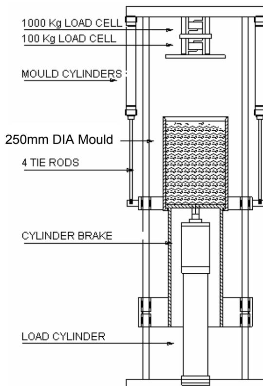
**Figure 2.9 Final version of schematic of the coal tester**
