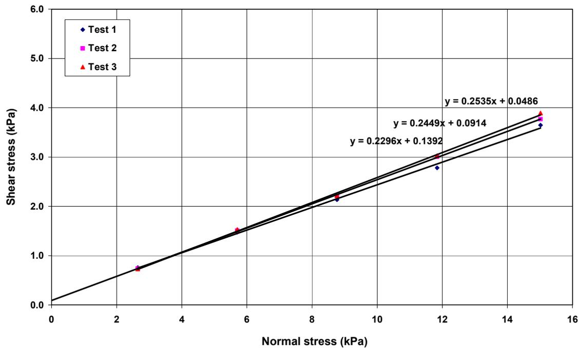
Figure 4.9 Shear stress vs. normal stress for wet coal on Mylar wall
