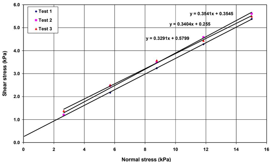
Figure 4.7 Shear stress vs. normal stress for wet coal on mild steel wall
