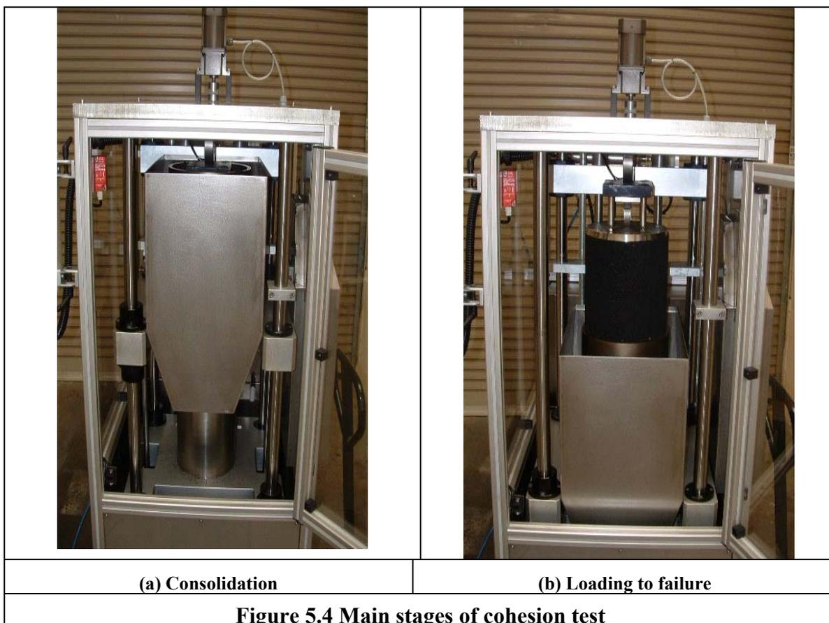
**Figure 5.4 Main stages of cohesion test**
