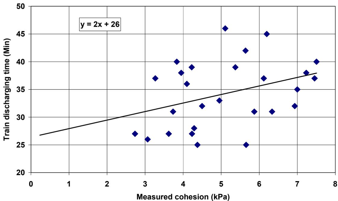
Figure 6.14 Train discharging time vs cohesion measured using AECT
