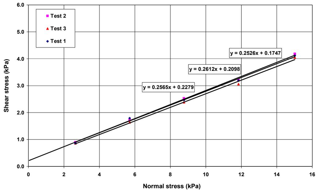
**Figure 4.4 Shear stress vs. normal stress for dry coal on nedox treated wall**
