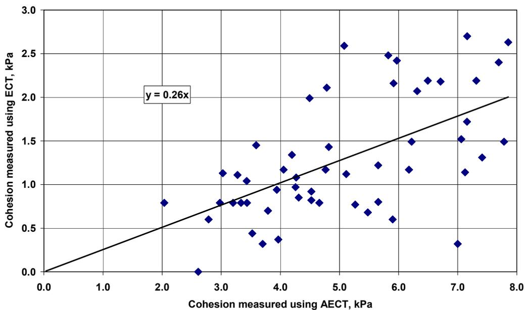
Figure 6.13 Comparison of cohesion values measured by ECT and AECT
