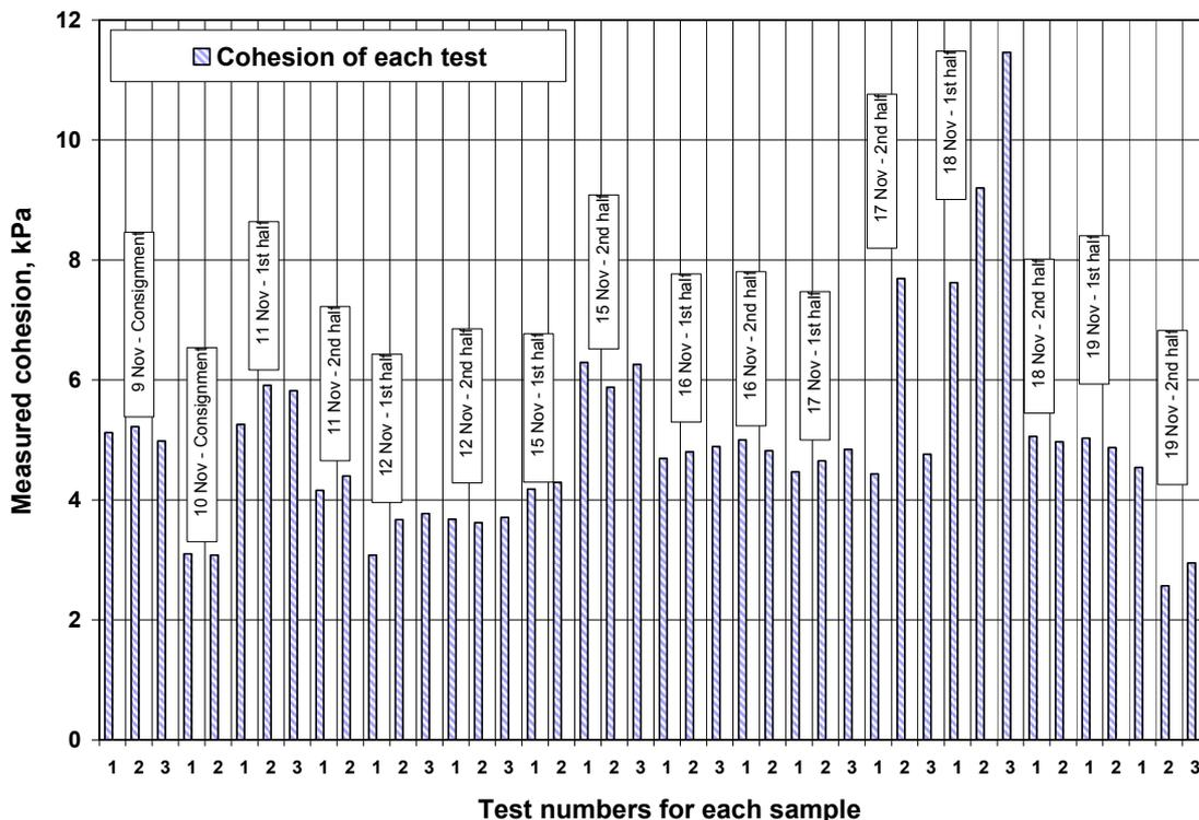
Figure 6.6 Measured cohesion during the trial period
